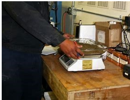
CSA A23.2-11A Test method for surface moisture in fine and coarse aggregate.
