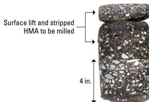
Figure 8.2. Core showing pavement that can be milled to remove stripped/unsound material, with 4 in. of HMA remaining in good condition
