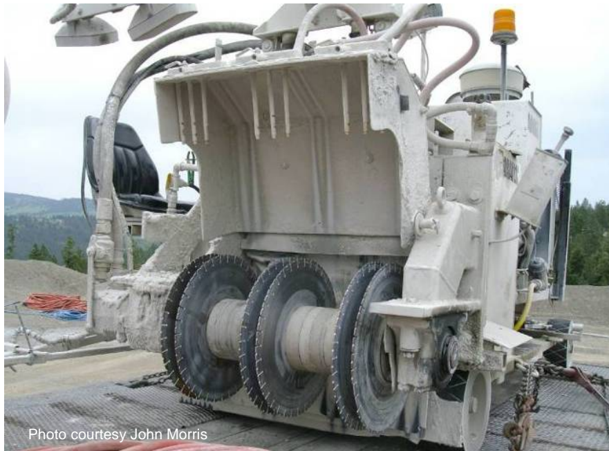
Figure 10 Diamond blades and spacing for three dowel bar slots per wheelpath.
