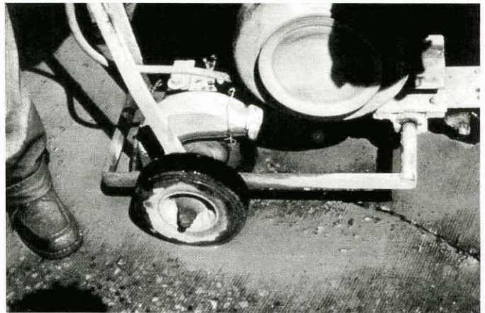
Figure 27 Crack sawing equipment. Note the small diameter blade and pivoting front wheel.
